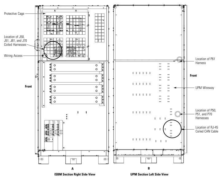
Figure 4-14. UPS Intercabinet Interface Harness Locations
